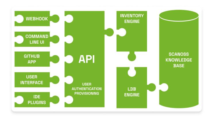
Client-side applications and middleware connect to the RESTful API via https. The API handles interaction with the Inventory Engine, which uses the LDB interfaces to query the database.
